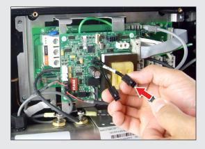
Insert the Balboa Wi-Fi Cable into the first end of the Y-Cable (25657) Panel Jack.
