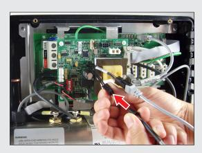
Insert your Control Panel into the second end of the Y-Cable Panel Jack.
