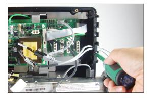
Insert the plastic holder and screw back in place. Make sure the 2 cable wires are secure in place.
