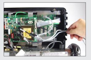
– Place the Wi-Fi cable and Control Panel cable inside the wire holder.
