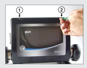
Use a phillips screwdriver to remove the 2 top screws that hold the system cover in place.
