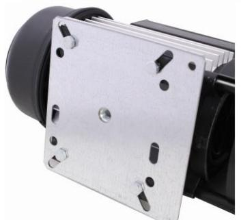
2. With a mounting plate, you simply screw one M10 bolt or a threaded pole up into the nut that is integrated in the plate, and the pump is in place.
