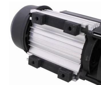
1. The easily accessible rubber feet allow quick installation of the pump, by screwing 4 pcs. of M6 bolts up into the nuts, that are integrated in the rubber feet.
